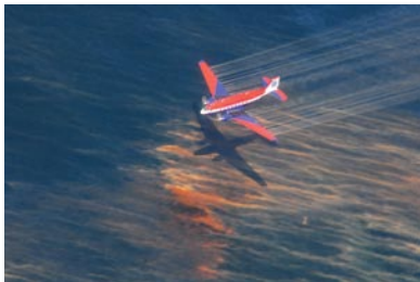
Aircraft applying chemical oil dispersant over an oil discharge.
